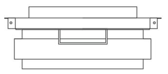
The Chute Hatch Door is manufactured from heavy grade steel 2.5mm thick with internal supports and the body of the unit is 3mm or 5mm thick steel and is removable so it can be re-placed if in any reason it has become compromised/damaged. Each unit is supplied with 450mm spigots round and square which are 5mm under sized so the chute ductwork will fit over the spigots. The units are then riveted or tech screwed to the chute ductwork.
